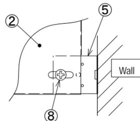
4. Make screw holes (diameter  $\phi 5/16$ ", with depth more than 1.6") using a drill to the wall and hammer the wall anchors⑩ into the screw holes. (If needed). (Fig.4)
