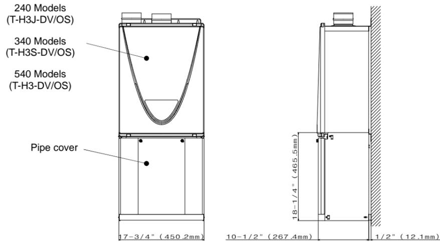
**NOTE:** This pipe cover is for the 240 Models (T-H3J-DV/OS), 340 Models (T-H3S-DV/OS), and 540 Models (T-H3-DV/OS).
