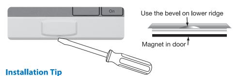
Gently slide a screwdriver into the bottom edge of the badge. Gently turn the screwdriver counter clockwise. The badge is held on by a magnet. The badge should pry off easily. Do not use force.
