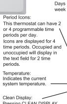
Pressing CLEAN DISPLAY will allow 30 seconds to clean the display. The keys will be inoperable during this time. CLEAN will appear if your contractor has programmed a filter change reminder. Press CLEAN when filter has been replaced to reset the filter change reminder timer.
