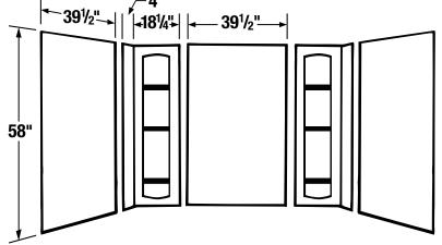
**General:** Furnish and install as shown on plans DURAWALL® Bathtub Walls, model 56, as manufactured by E.L. Mustee & Sons, Inc. The deluxe hi-impact Co/Poly wall system shall be five-piece construction with six formed shelves, and one-piece, seamless corner panels with overlapping edges and have uniform color throughout entire thickness. Color \_\_\_\_\_\_ (White, Bone).
