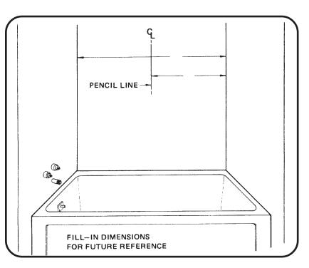
2. Accurately measure tub spout and handle(s) hole location on alcove side wall and transfer dimensions to one of the remaining flat panels. You may want to make a template (use shipping carton) to check hole layout before you cut holes into side panel. After you have double checked your measurements, using the proper size drill or hole saw, cut out holes for outlets.
