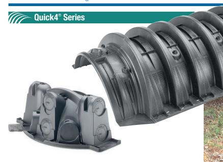
The Quick4® Standard Chamber fits in a 36" wide trench and is ideal for curved or straight systems. It features the patent-pending Contour Swivel Connection™ which permits turns up to 15°, right or left. The MultiPort™ endcap allows multiple piping options and eliminates pipe fittings. The chamber's four-foot length provides optimal installation flexibility.
