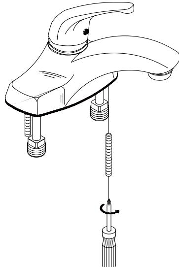
3. Place silicone sealant beneath the plastic gasket and install the faucet through the center hole.
