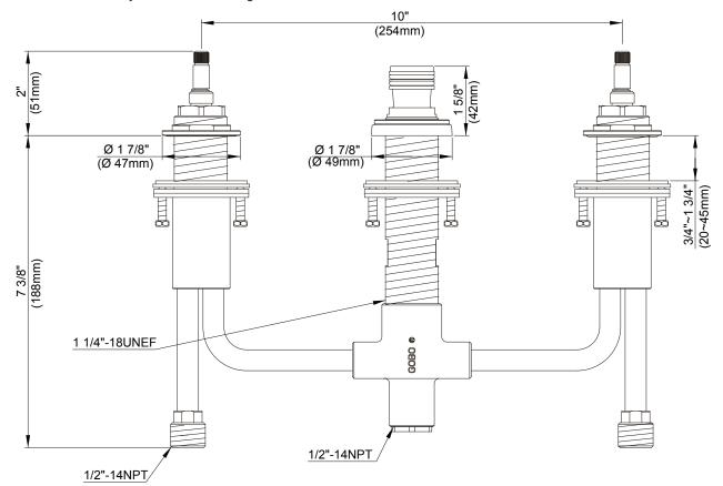
\* Installation method shown is for deck thickness of less than 1-3/4". If the installation is for deck thickness between 1-3/4" and 3-1/2", the sleeve nut needs to be reversed.
