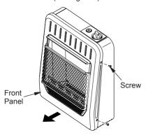
Figure 5 - Removing Front Panel Of Heater
