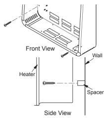
Figure 10 - Installing Bottom Mounting Screws
