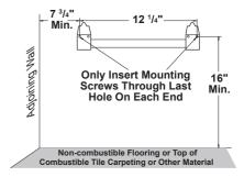
Figure 6 - Mounting Bracket Clearances
