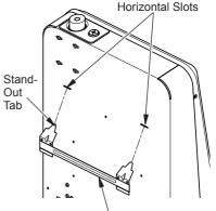
Mounting Bracket (attached to wall)
