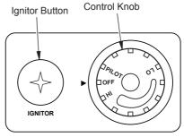
Figure 18 - Control Knob in the OFF Position
