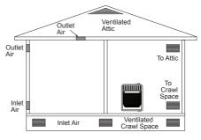
Figure 3 - Ventilation Air from Outdoors
