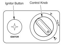
Figure 16 - Control Knob in the OFF Position
