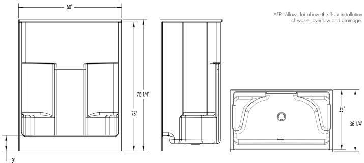
FEATURES Ibs (kg) Dimensional Tolerance ± %". Dimensions needed for site preparation should be measured from the unit. Aquatic assumes no responsibility for preparatory work.
